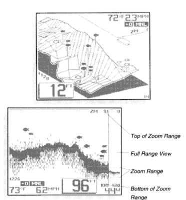
To enable Zoom, adjust the horizontal lines to the depth of the zoom range using the UP and DOWN arrow buttons, then enable Zoom using the ENTER button.
